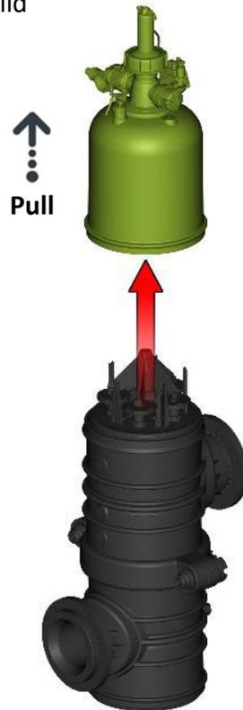
8. Pull up and remove the bridge according to the following steps:
