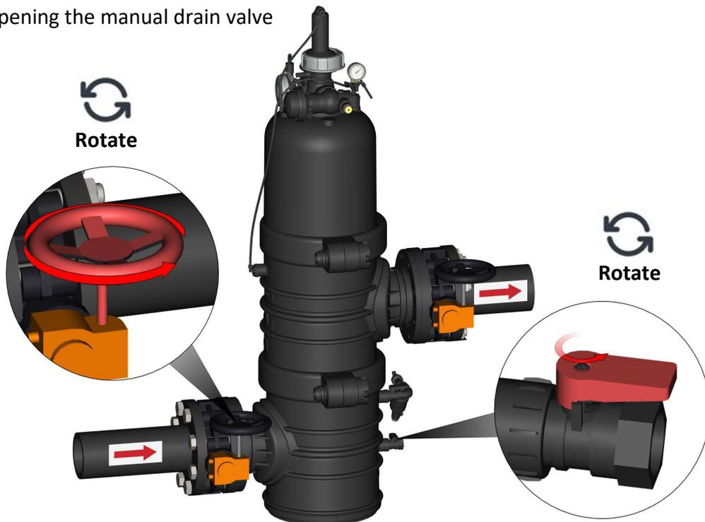
4. Make sure that the pressure gauge is on zero!
