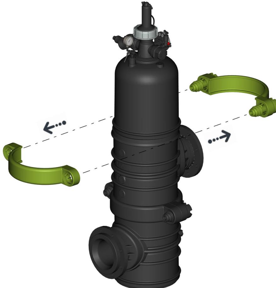
7. Pull up and remove the filter's lid
