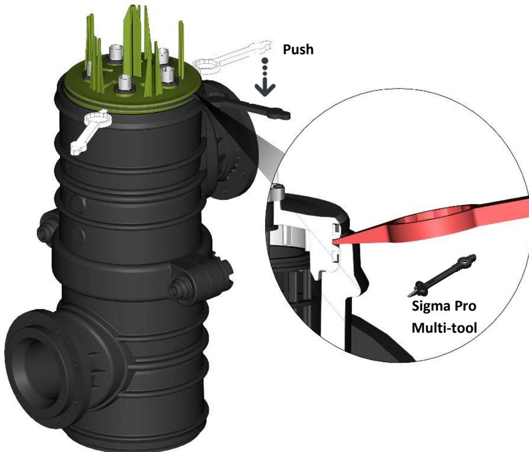
c. Remove suction-scanner's top plate
