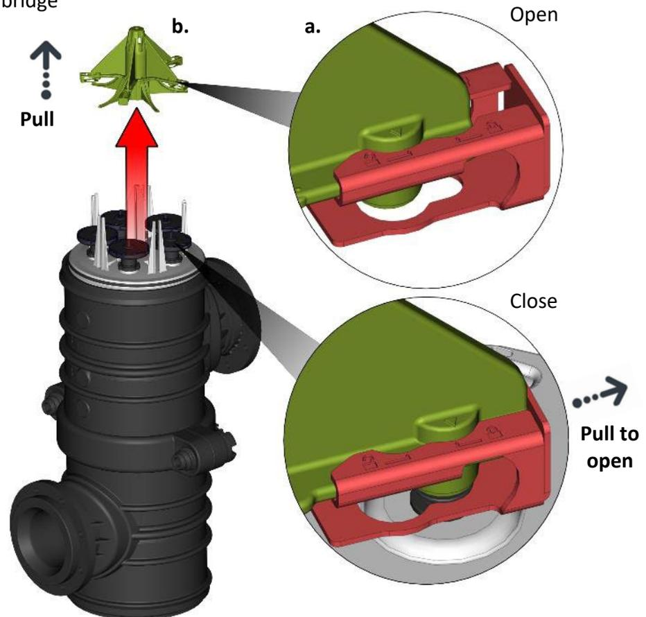
9. Remove the turbine from the five suction-scanner's upper shaft
