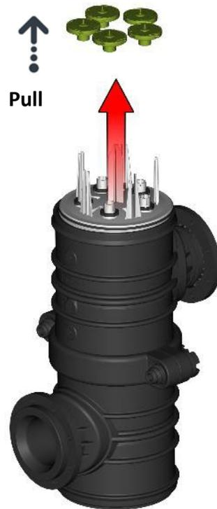
10. Remove the suction-scanner's top plate:
