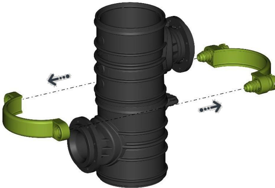
4. Lift and rotate the Sigma body and plate to the desired position
