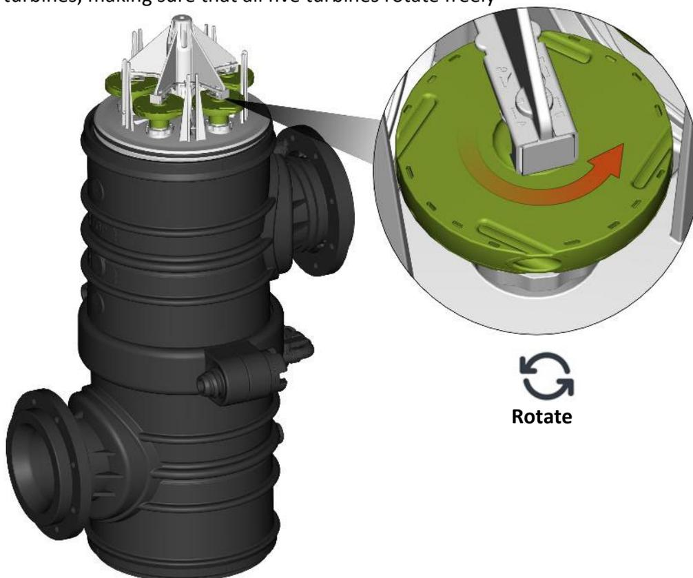
7. Lift the bridge up and down to make sure all turbines connect to the bridge and the scanners move freely
