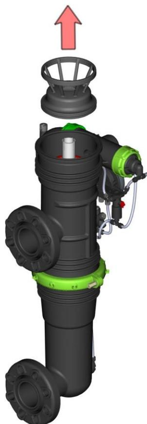
5. Remove the scanner and nozzles
