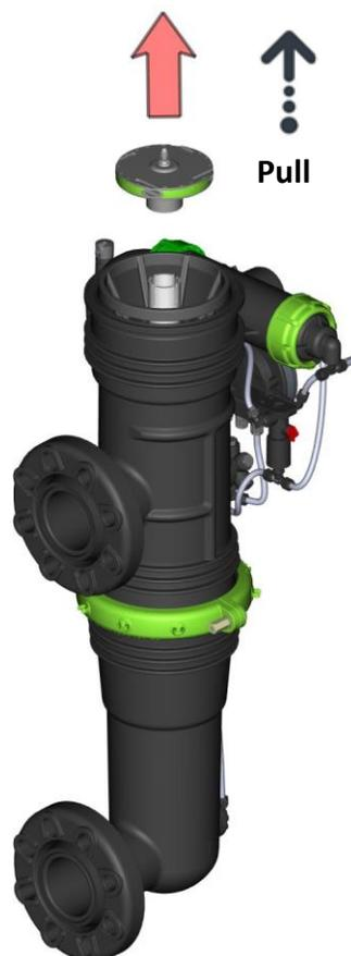
4. Remove the separation plate
