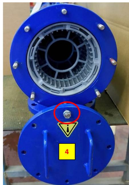
4. Pull the coarse screen out of the filter housing.
