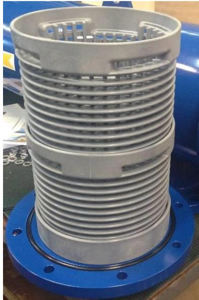
5. Pull the fine screen out of the filter housing. If it is difficult to release the screens use Amiad's Push Pull Tool (Catalog Number 7001900-001985) to extract the screen by performing the following procedure:
