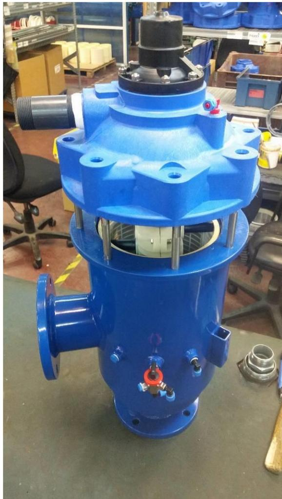
3. Using the special tool, pull the screen out of the housing. (CAT. NO. 710103-001121- TOOL EXTRACTOR M100 S/ST304 F/FINE SCREEN)
